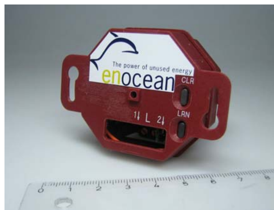
Figure 14: The total switching receiver electronics fits into a standard in-wall unit (PPS and SPS power supplies, TCM radio module, bi-stable switching relay)
