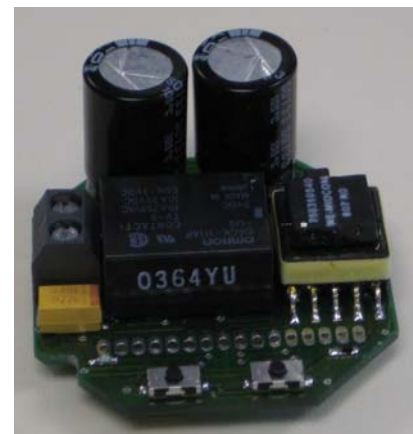
Figure 9: Connecting diagram and prototype of the high efficiency EnOcean SPS
