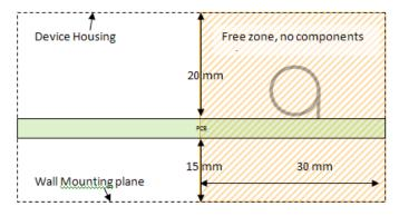
Fig. 7 Antenna positioning within housing
