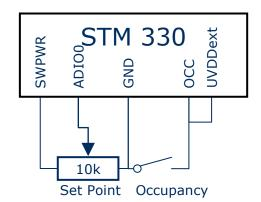
With default settings the module wakes up every 100s and transmits a life signal every 15 min. In addition, a wake up can be triggered externally using an external occupancy button or the internal LRN button.
