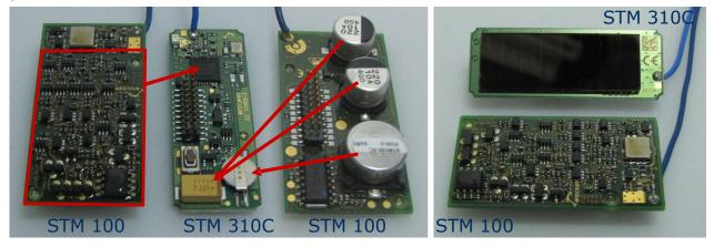
Due to the much higher level of integration the back side of the module could be emptied completely making room for a solar cell directly mounted onto the module.
