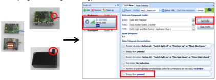
Remark: In order to send EnOcean standard radio telegrams according to the EEP specification, you need to set the right contact pins on PTM 330. Without doing this PTM 330 can't control a standard receiver/actuator. For details see PTM 330 user manual.
