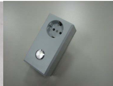
Fig. 3: Line powered radio controller
