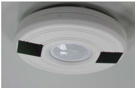
Fig. 1: Ambient light powered Motion Sensor
