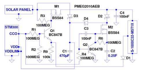
**Charge switcher** is the PMOS transistor M1, driven from the STM 300 charge control output CCO/WXODIO over Q1. To start with, as long as the Vdd voltage is below the Von threshold, only the small storage C1 is filled over D3. Once the threshold is reached, the charge control signal CCO goes high, Q2 and M2 are turned on and the longterm storage C2 is filled over M2.
