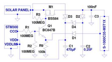
This circuit implements only charge with overvoltage protection but without undervoltage protection. It is actually the basic circuit above extended with overvoltage protection. The circuit can be used for standard longterm storage not requiring undervoltage protection but having a limited nominal voltage, below 5 V. As mentioned, this circuit cannot avoid longterm deep storage discharging, meaning a longer recovery time.
